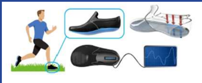
Fig. 1. Schematic representation of the flexothermoelectric device
