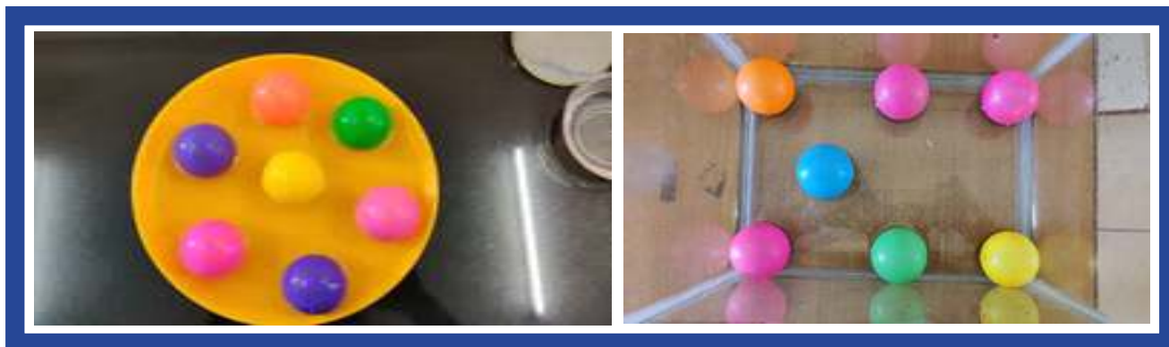
Fig. 1(a) Hexagon symmetry in a circular tray and (b) Cubic arrangement with defect in rectangle tray.
